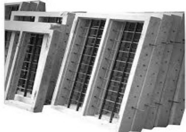
Fig. 6: RCC Window Frames
